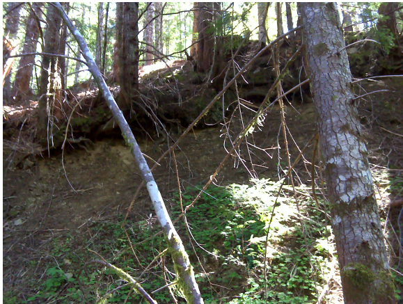
A-16-6C N47 35.282 W123 57.992 Notes: mass wasting undercutting undercutting trees on underside of road; creating conduit for water Direction: 20°
